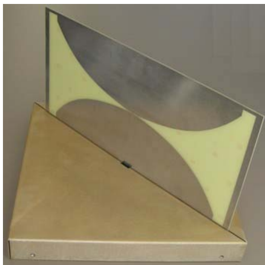
Fig. 7 Photograph of a prototype of the vehicle mount profile optimized slot
