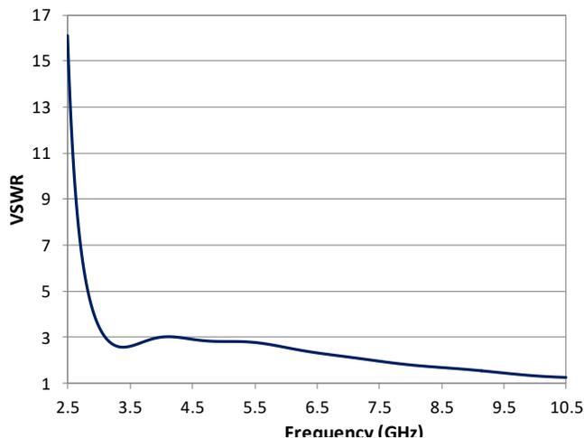
Fig. 2. Predicted VSWR of BW UWB Antenna.
