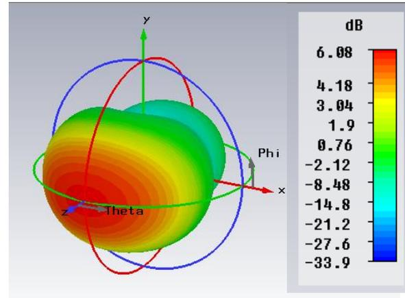
Fig. 3. Predicted radiation performance of BW UWB antenna at 3 GHz.
