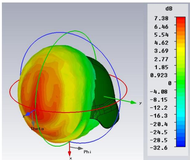
Fig. 10. Predicted radiation performance of BW UWB antenna on helmet at 6 GHz.
