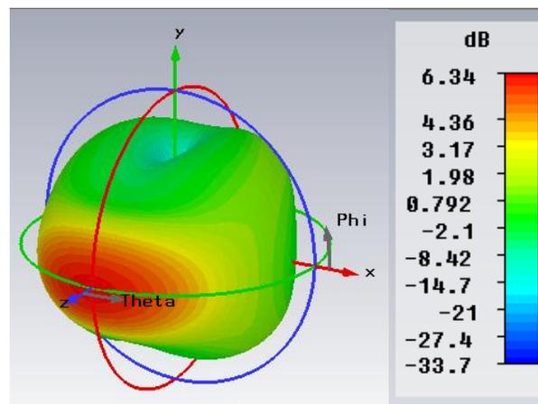
Fig. 5. Predicted radiation performance of BW UWB antenna at 10 GHz.
