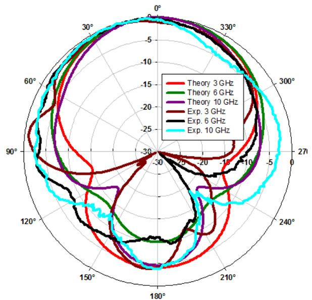
Fig. 8. Measured azimuth radiation patterns of BW UWB antenna.
