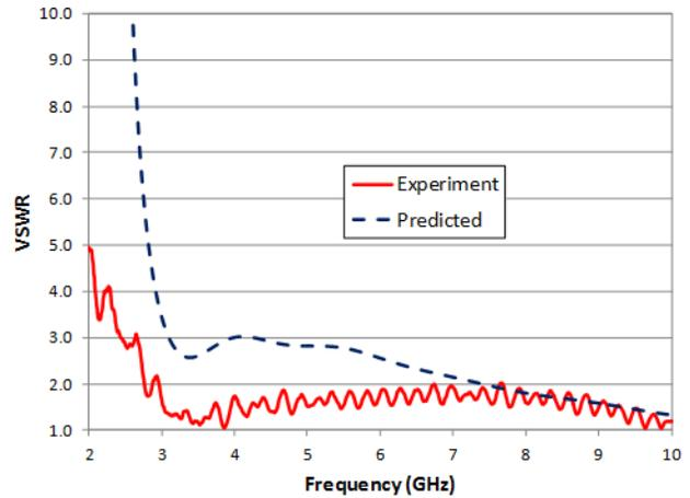
Fig. 7. VSWR of BW UWB antenna.
