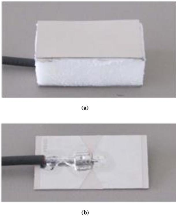
Fig. 6. Photograph of: (a) BW UWB antenna; (b) cable feed.
