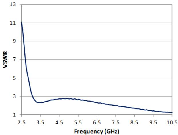
Fig. 9. Predicted VSWR of BW UWB antenna when mounted on a helmet.
