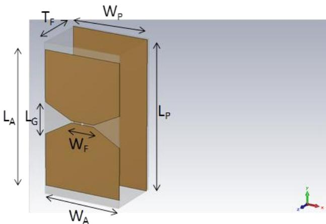
Fig. 1. Schematic of wideband antenna. Dimensions:  $L_A = 34$  mm,  $W_A = 20$  mm,  $L_P = 38$  mm,  $W_P = 20$  mm,  $T_F = 14$  mm,  $W_F = 7$  mm,  $L_G = 8$  mm
