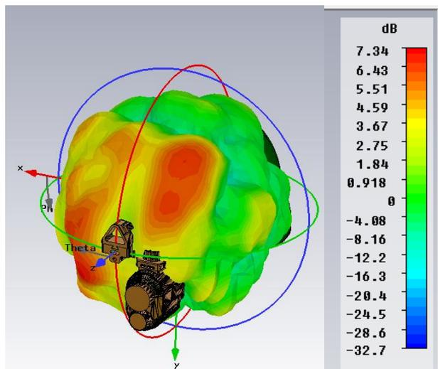
Fig. 11. Predicted radiation performance of BW UWB antenna on helmet in presence of viewer and horn at 6 GHz.
