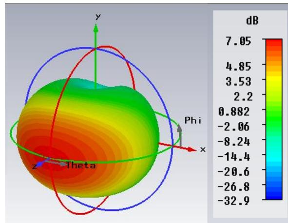
Fig. 4. Predicted radiation performance of BW UWB antenna at 6 GHz.
