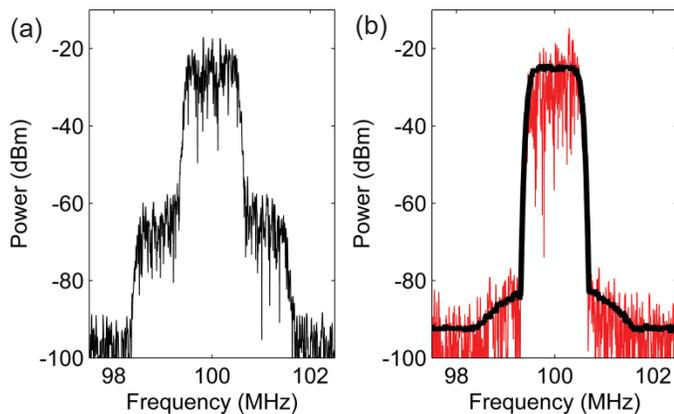
Fig. 4. (a) Original output. (b) Digitally linearized output with overlay of original input signal (black line).
