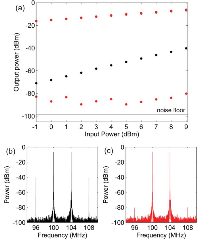
Fig. 2. (a) Plot of IMD3 and fundamental output power versus input power. Black: Original output. Red: Digitally linearized output. (b) Original two tone spectrum for input power of 9 dBm (c) Digitally linearized spectrum for input power of 9 dBm.
