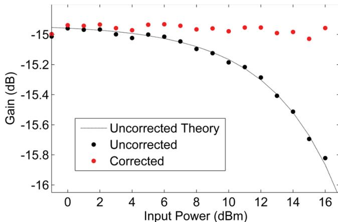
Fig. 3. Gain compression of the link before and after digital linearization.
