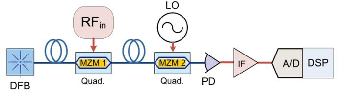
Fig. 1. Experimental setup. All fiber is polarization-maintaining. Abbreviations: DFB: distributed feedback laser, MZM: Mach-Zehnder modulator, Quad: quadrature, PD: photodiode, A/D: analog-to-digital converter, DSP: digital signal processing.
