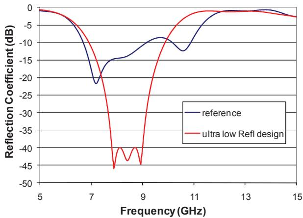
Fig. 2. Comparison of reflection coefficient of ASP antennas.
