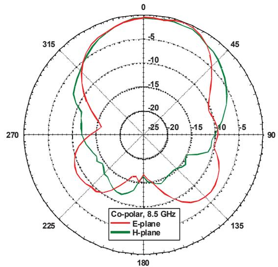
Fig. 4. Measured radiation patterns of low reflection coefficient ASP antenna at 8.5 GHz.
